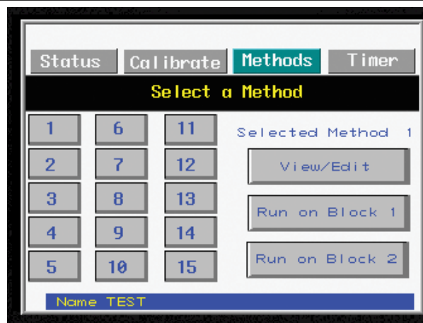
Figure 1. Selecting Method from the main menu will take you to the screen shown above (Figure 1). Click on the Method Number you wish to program.
