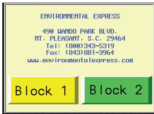
The first screen to appear when you turn on your block gives you the option of choosing Block 1 or Block 2. Choosing either block will take you to the STATUS screen.
