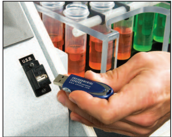
The controller logs and records all digestion procedures, step by step. Data can easily be transferred to a PC or other back up device via the USB port.
