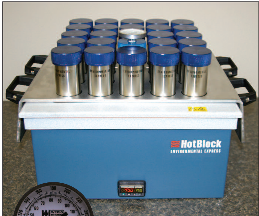
A Soil Extraction Reference Cell monitors and displays the internal temperature of the solvent during the extraction process.
