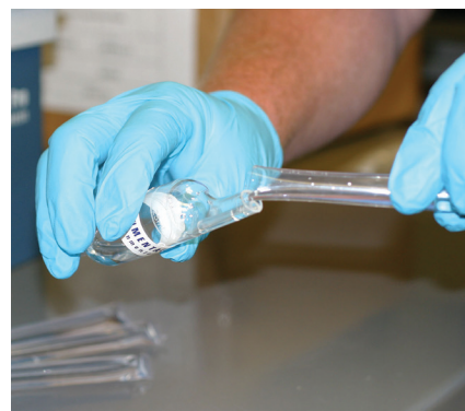
Pour the entire 5mL concentrate into the SimpleDist collection trap.
