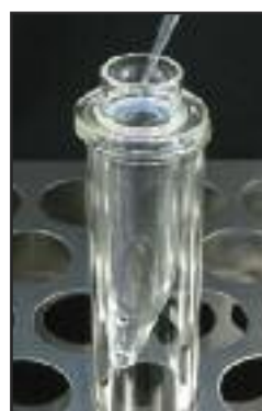
Splash-head tube inserts ensure safe reagent addition to digestion tubes during the digestion process.
