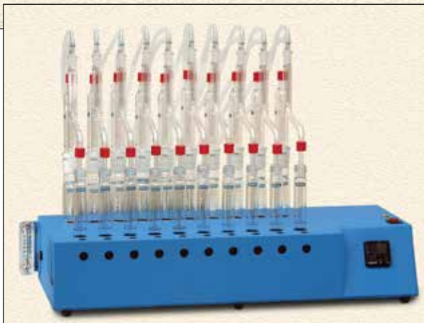
MicroBlock-R System shown with ammonia glassware
